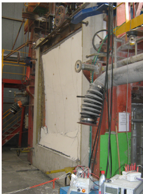
Photo A (up) Unexposed side before the test Photo B (down) Breaking of the wall (112 th minute).
